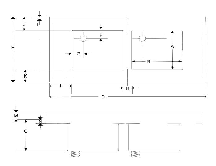
This unit is designed with marine edge on horizontal surfaces to avoid countertop spilling and a backsplash unit. Uniquely designed one piece molding with integral sink outlets, edge and backsplash. Unit has attached 1-1/8" plywood for easy affixing to any counter or cabinet top unit. Standard color is non-glare black.
