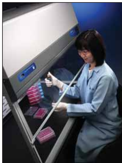
Figure 4. The Purifier Class I Safety Enclosure protects the user, but not the product, from airborne particulates.
