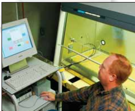
Figure 6. Prior to shipment, the proper airflow in the Purifier Delta Series Cabinet is verified.
