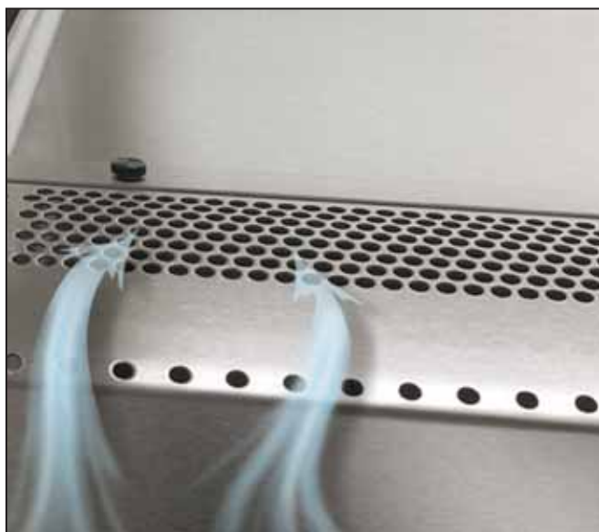
Reserve-Air™ Secondary Airflow Slots, located in front of the air foil's inflow grille, draw air into the Purifier should the operator inadvertently block the grille area. Safe airflow is always maintained.
