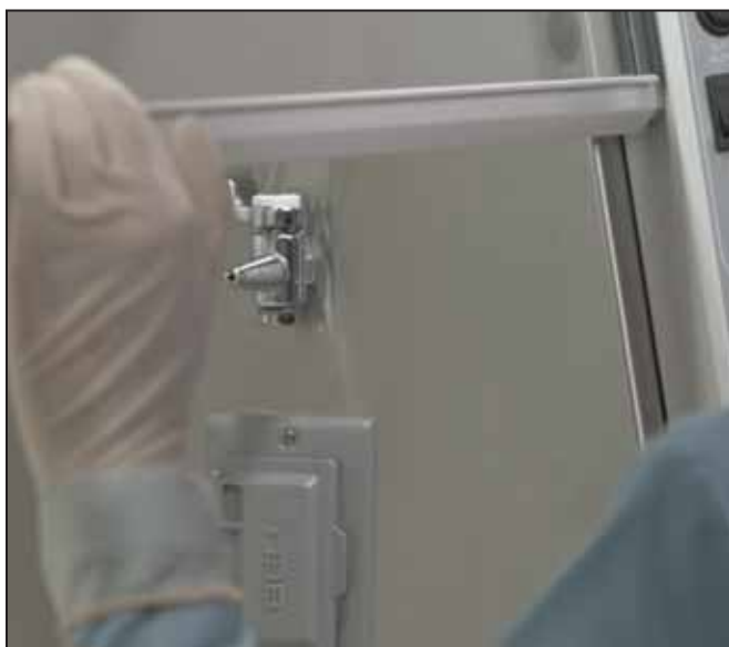
The sash is counterweighted for balance, greater reliability and durability. The anti-racking mechanism ensures easy raising and lowering from all areas of the sash handle.
