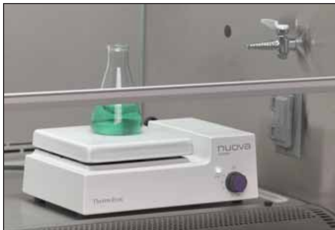
Service fixtures are mounted within reach of the operator but somewhat higher so that they are less likely to snag on clothing or bump the user's forearms.
