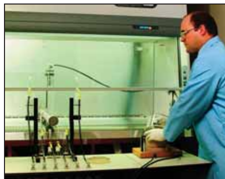
Figure 5. A Labconco engineer sets up equipment in a Purifier Delta Series Class II Cabinet to conduct a biological challenge test.
