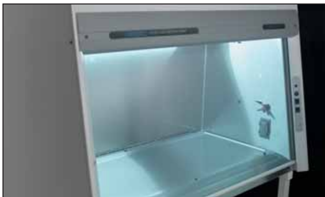
The angled sash may be completely closed when not in use, providing a physical barrier.
