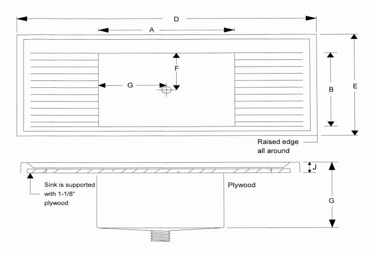
One piece molded sink (with integral molded 1-1/2" tail piece) countertop unit with pitched ribbed drainboards and 1-1/8" marine edge. Rear deck allows for mounting water fixtures.
